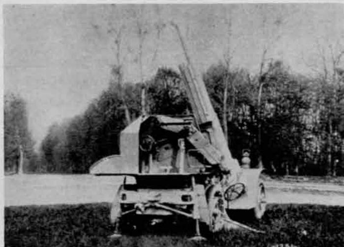
Fig. 1—75mm AA autocannon mounted on truck (French).
